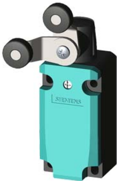
SIRIUS POSITION SWITCH METAL ENCLOSURE 40MM TO EN50041 DEVICE CONNECTION 1X (M20X1.5) 1NO/ 1NC SNAP-ACTION CONTACTS FORK LEVER ACTUATOR W. METAL LEVER AND PLASTIC ROLLERS 19MM
