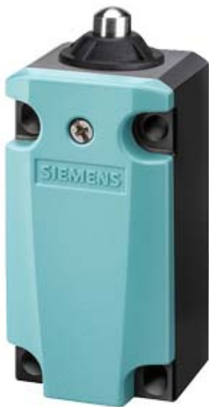
SIRIUS POSITION SWITCH METAL ENCLOSURE 40MM TO EN50041 DEVICE CONNECTION 1X (M20X1.5) 1NO/ 2NC SLOW-ACTION CONTACTS PLAIN PLUNGER, STAINLESS STEEL
