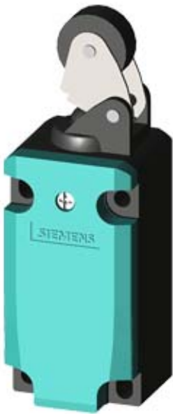
SIRIUS POSITION SWITCH METAL ENCLOSURE 40MM TO EN50041 DEVICE CONNECTION 1X (M20X1.5) 1NO/ 2NC SLOW-ACTION CONTACTS METAL ROLLER LEVER AND PLASTIC ROLLER 22MM
