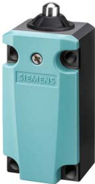
SIRIUS POSITION SWITCH METAL ENCLOSURE 40MM TO EN50041 DEVICE CONNECTION 1X (M20X1.5) 1NO/ 2NC SNAP-ACTION CONTACTS PLAIN PLUNGER, STAINLESS STEEL
