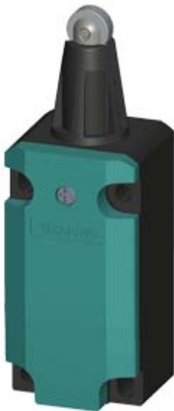
SIRIUS POSITION SWITCH METAL ENCLOSURE 40MM TO EN50041 DEVICE CONNECTION 1X (M20X1.5) 1NO/ 2NC SNAP-ACTION CONTACTS ROLLER PLUNGER W. STAINLESS STEEL ROLLER 13MM
