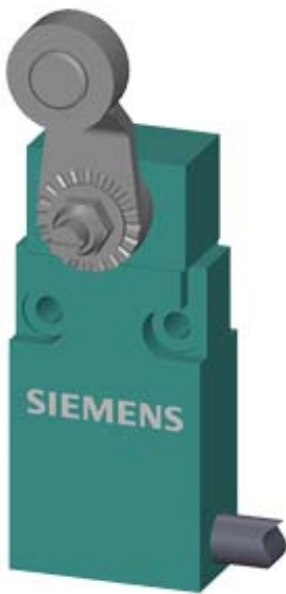
COMPACT SWITCH 30MM WIDE W. CONNECTING CABLE 2M SNAP-ACTION CONTACTS 1NO+1NC TWIST LEVER
