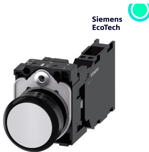
Pushbutton, 22 mm, round, plastic, white, pushbutton, flat, momentary contact type, with holder 1 NO+1 NC, spring-type terminal, with laser labeling, lower case
