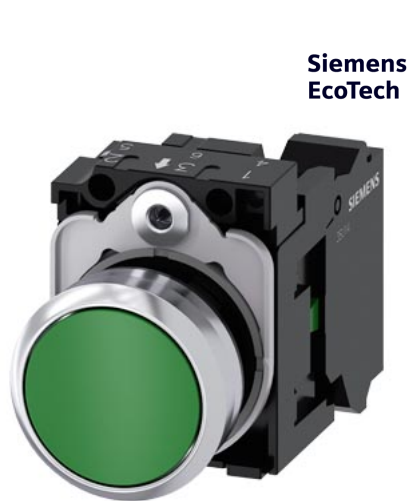
Pushbutton, 22 mm, round, metal, shiny, green, pushbutton, flat, momentary contact type, 1 NO, spring-type terminal, with laser labeling, upper case
