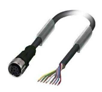
CABLE, 8-PIN, FREE CABLE END 10M LONG, FOR RFID SAFETY SWITCH 3SE63, ON STRAIGHT SOCKET M12, FOR 2A AND 30V
