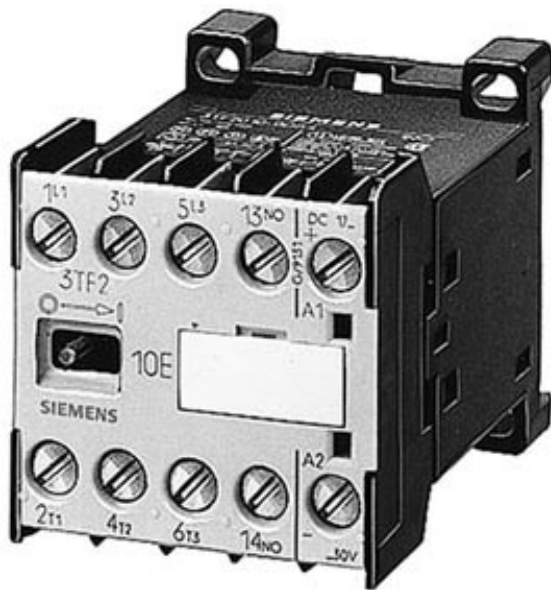
CONTACTOR, SIZE 00, 3-POLE AC-3, 4KW/400V, SCREW TERMINALS AUXILIARY CONTACT 10E (1NO) DC SOLENOID SYSTEM DC 220V
