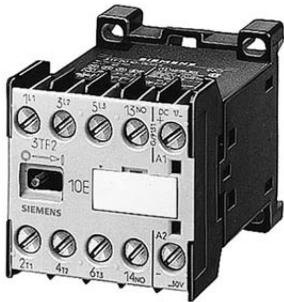
CONTACTOR,SIZE 00, 3-POLE AC-3, 4KW/400V,SCREW CONNECTION AUXILIARY CONTACTS 22E(2NO+2NC) WIDTH 45MM DC SOLENOID SYSTEM DC 24V
