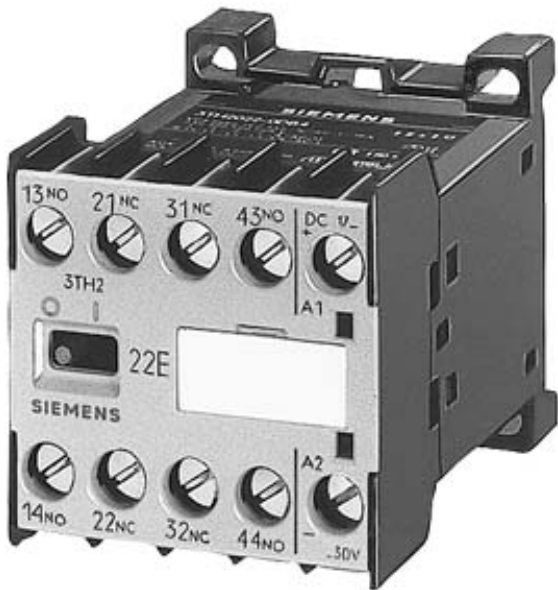
CONTACTOR RELAY 22E EN 50 011 2NO+2NC, SCREW TERMINALS AC OPERATION AC 60HZ 110V/50HZ 92V
