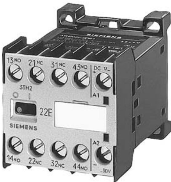
CONTACTOR RELAY 22E EN 50 011 2NO+2NC, SCREW TERMINALS AC OPERATION AC 60HZ 120V/50HZ 100V
