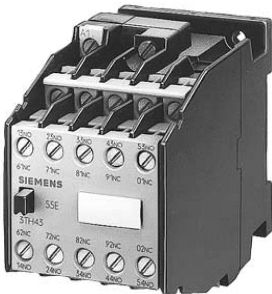
CONTACTOR RELAY 73E EN 50 011 7NO+3NC, TAB CONNECTOR AC OPERATION AC 50HZ 110V/60HZ 132V
