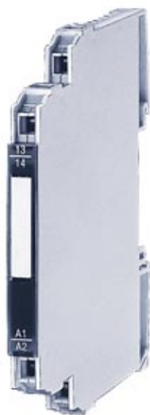
INPUT COUPLER WITH PLUGGABLE RELAY, 1 CHANGE OV. GOLD-PLATED SPRING-LOADED TERMINAL 115 V AC/DC CASING WIDTH 6.2 MM
