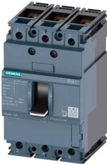
CIRCUIT BREAKER 3VA1 IEC FRAME 100 BREAKING CAPACITY CLASS B ICU=16KA @ 415 V 3-POLE, LINE PROTECTION TM210, FTFM, IN=63A OVERLOAD PROTECTION IR=63A FIXED SHORT CIRCUIT PROTECTION II=10 X IN BUSBAR CONNECTION UNDERVOLTAGE RELEASE (UVR) 120-127 V AC 50/60 HZ 2 AUXILIARY SWITCH HQ 1 TRIP ALARM SWITCH HQ
