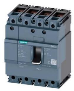
SWITCH DISCONNECTOR 3VA1 IEC FRAME 160 4-POLE SD100, IN=63A WITHOUT OVERLOAD PROTECTION WITHOUT SHORT CIRCUIT PROT. BUSBAR CONNECTION SHUNT TRIP (STL) 220-250 V DC, 208-277 V AC 2 AUXILIARY SWITCH HQ 1 TRIP ALARM SWITCH HQ
