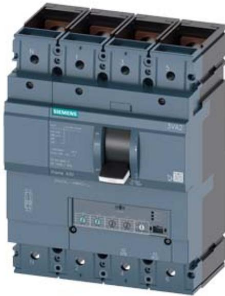
CIRCUIT BREAKER 3VA2 IEC FRAME 630 BREAKING CAPACITY CLASS C ICU=110KA @ 415 V 4-POLE, LINE PROTECTION ETU330, LIG, IN=400A OVERLOAD PROTECTION IR=160A ...400A SHORT CIRCUIT PROTECTION II=1,5...12 X IN NEUTRAL PROTECTION ADJUSTABLE(OFF,50%,100%) GROUND-FAULT-PROTECTION IG=0,2... 1 X IN, TG=0,1/0,3S BUSBAR CONNECTION
