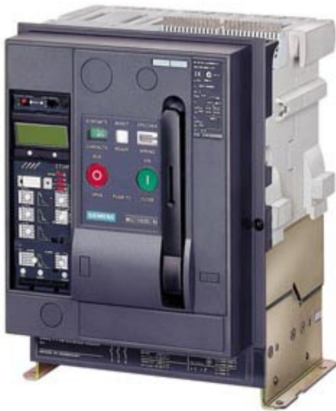
FIXED-MOUNTED CIRCUIT BREAKER 4-POLE, SIZE I, IEC IN=1000A TO 690V, AC50/60HZ ICU=55KA AT 500V REAR CONNECTION HORIZONTAL
