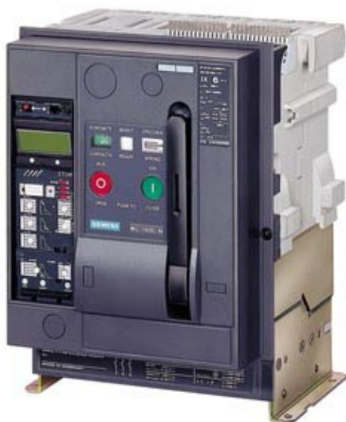
FIXED-MOUNTED CIRCUIT BREAKER 4-POLE, SIZE I, IEC IN=1000A TO 690V, AC50/60HZ ICU=66KA AT 500V REAR CONNECTION HORIZONTAL
