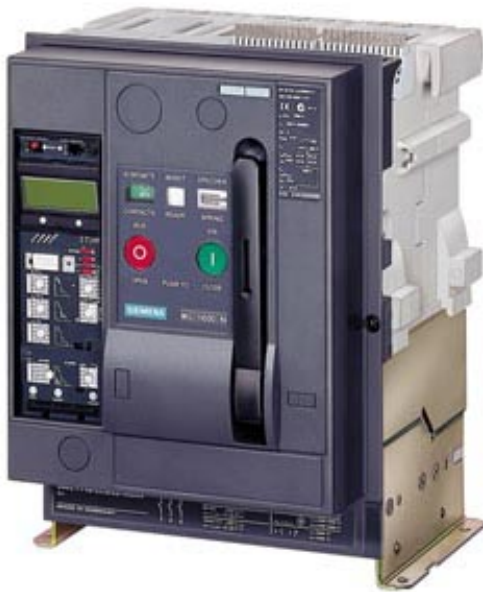
FIXED-MOUNTED CIRCUIT BREAKER 3-POLE, SIZE I, IEC IN=1250A TO 690V, AC50/60HZ ICU=55KA AT 500V FRNT.CONN. TOP/BOT. SINGLE-HOLE
