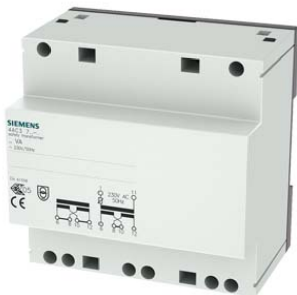
SAFETY TRANSFORMER, 40VA PRIM 230V AC,50HZ, SEK 2X12V / 24V AC WITH PTC PROT.,5MW
