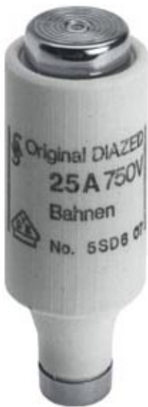
DIAZED FUSE-LINK 750V DC RAILROAD PROPERTY PROTECTION CHARACTERISTICS FAST ACTING SIZE DIII, E33, 25A
