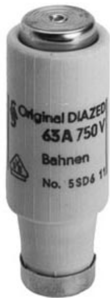
DIAZED FUSE-LINK 750V DC RAILROAD PROPERTY PROTECTION CHARACTERISTICS FAST ACTING SIZE DIII, E33, 50A
