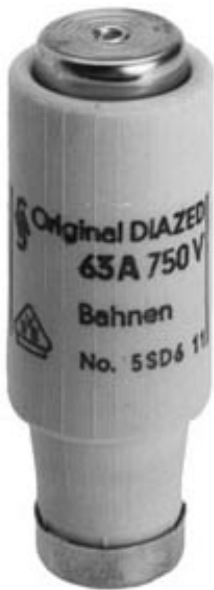
DIAZED FUSE-LINK 750V DC RAILROAD PROPERTY PROTECTION CHARACTERISTICS FAST ACTING SIZE DIII, E33, 63A
