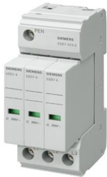
SURGE ARRESTER TYPE 2 REQUIREMENT CATEGORY C, UC 350V PLUG-IN PROTECTION BLOCKS 3-POLE, 3+0 CIRCUIT FOR TNC SYSTEMS NARROW DESIGN
