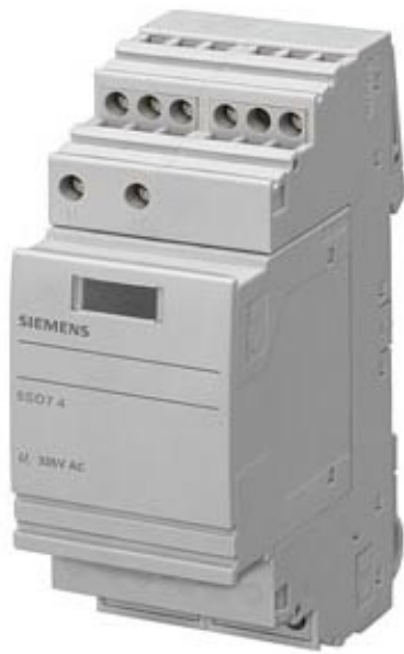
SURGE ARRESTER TYPE 3 REQUIREMENT CATEGORY D RATED VOLTAGE UN 230V UC DC275V/AC253V, 4POLE FOR 3PHASE POWER SUPPLY
