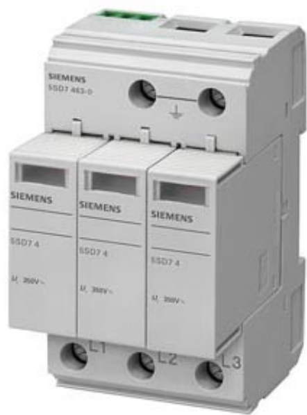
SURGE ARRESTER TYPE 2 REQUIREMENT CATEGORY C, UC 350V PLUG-IN PROTECTION BLOCKS 3-POLE, 3+0 CIRCUIT FOR TNC SYSTEMS
