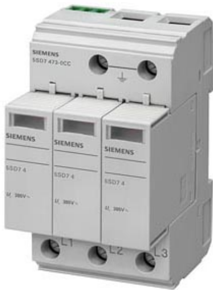
SURGE ARRESTER TYPE 2 REQUIREMENT CAT. C,UC 580V AC PROTECTION BLOCKS PLUGGABLE 3POLES, 3+0 CIRCUIT FOR IT SYSTEMS WITHOUT N CONDUCTOR
