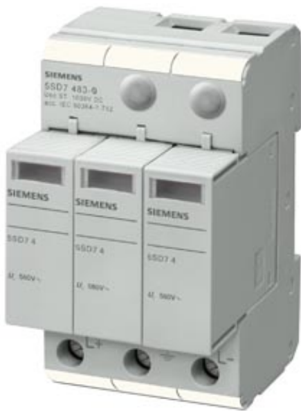
SURGE ARRESTER TYPE 2 CAT. C, UOC STC 1000V DC PROTECTION BLOCKS PLUGGABLE FOR PHOTOVOLTAICS
