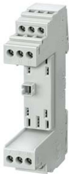
BASE ELEMENT 2X2, DIN RAIL 2 CHANNELS, 4 WIRES MOUNTING FOOT INDIRECT EARTHED VIA A GAS_FILLED SURGE ARRESTER FOR PLUGGING MODULE 5SD7522-. AND 5SD7550-4
