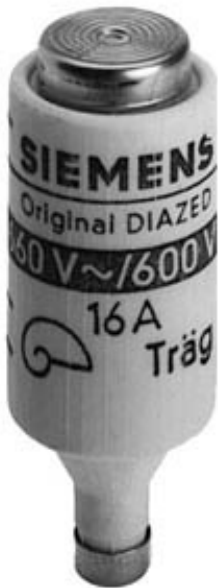
DIAZED FUSE-LINK 690V FOR CABLE AND LINE PROTECTION UTILIZATION CATEGORY GG SIZE DIII, E33, 16A
