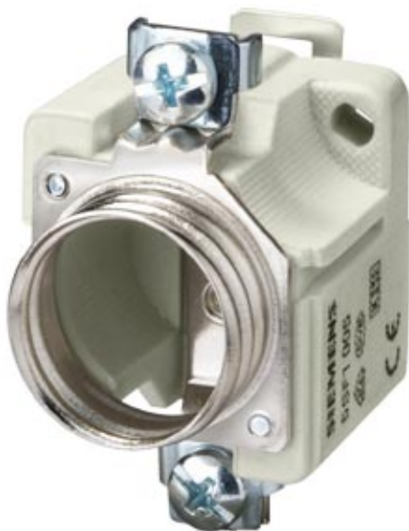
DIAZED-BASE DIII 63A AC690V DC500V SADDLE/SADDLE TERMINAL
