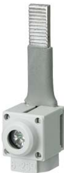
CONNECTION TERMINAL 25SQMM PIN-TYPE VERSION WITH BACK-SIDE ISOLATION WIRE-INFEED STRAIGHT
