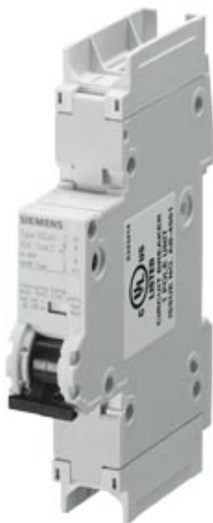
CIRCUIT BREAKER 240V 14KA, 1-POLE, C, 8A, D=70MM ACC. TO UL 489
