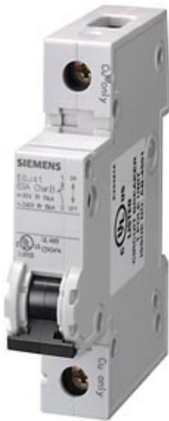
CIRCUIT BREAKER 240V 14KA, 1-POLE, B, 35A, D=70MM ACC. TO UL 489, SAME POLARITY
