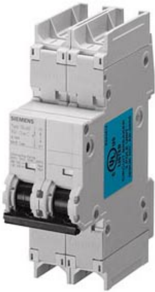
CIRCUIT BREAKER 240V 14KA, 2-POLE, D, 8A, D=70MM ACC. TO UL 489
