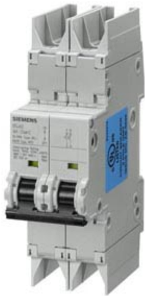
CIRCUIT BREAKER 10KA, 2POLE, D, 10A ACC. TO UL 489 - 480Y/277V
