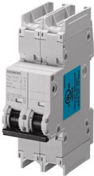
CIRCUIT BREAKER 240V 14KA, 2-POLE, C, 20A, D=70MM ACC. TO UL 489
