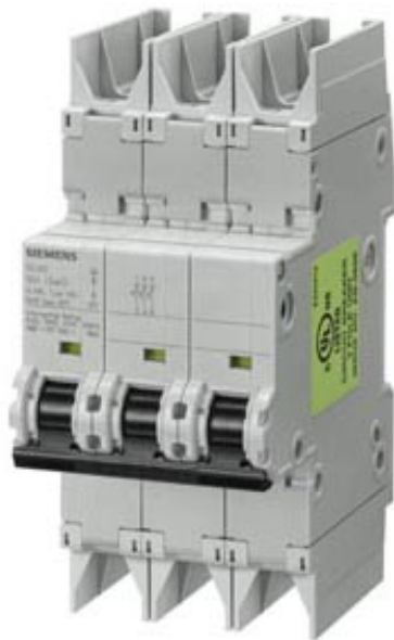
CIRCUIT BREAKER 10KA, 3POLE, C, 3A ACC. TO UL 489 - 480Y/277V
