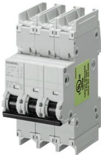
CIRCUIT BREAKER 240V 14KA, 3-POLE, D, 0,3A, D=70MM ACC. TO UL 489
