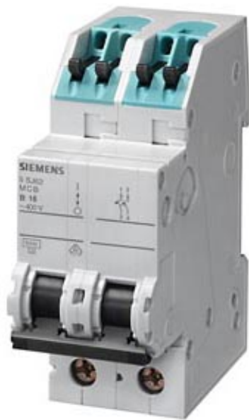
CIRCUIT BREAKER 230V 6KA, 1+N-POLE, B, 20A, D=70MM WITH SCREWLESS TAP-OFF TERMINAL
