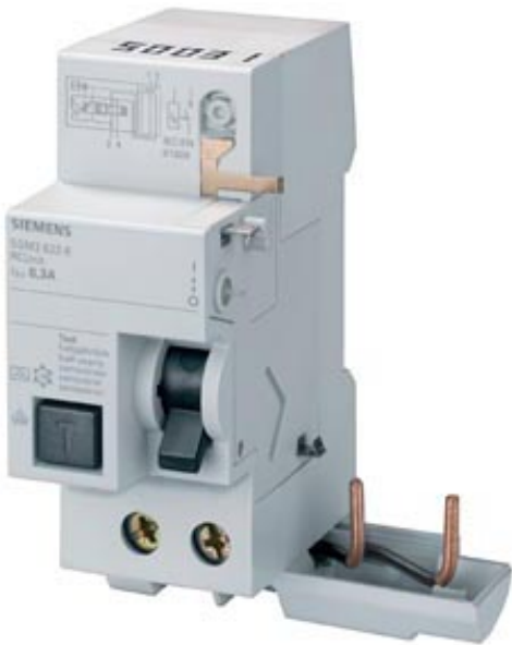
RC UNIT FOR MCB 5SY TYPE A (PSE/SSF), T=70 MM 0.3-63 A 2-POLE IFN 0.5 A 230 V
