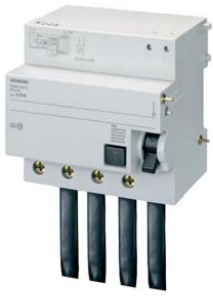
RC UNIT FOR MCB 5SX6+7 TYPE A (PSE/SSF), DEPTH=70MM 80/100A 4 POLE IFN 1A 400V FOR SELECTIVE SWITCH OFF
