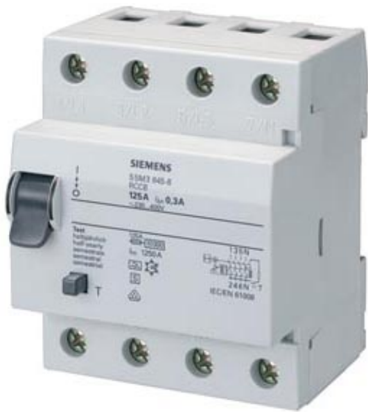
RES.CURRENT OP.CIRCUIT BREAKER TYPE A PSE/SSF 125A 3+N-POL IFN 300MA 400V 4MW FOR SELECTIVE SWITCH OFF
