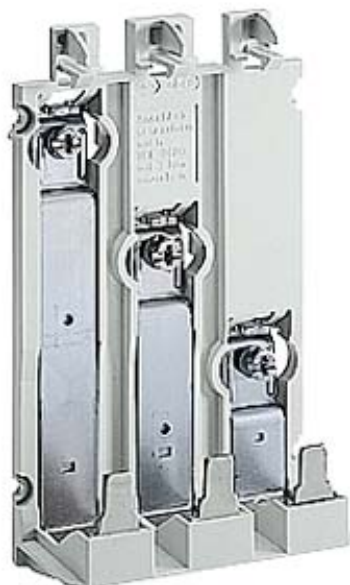
BUS BAR ADAPTER F.MAIN CIRCUIT BREAKER (SHU), FOR SNATCHING ON 40MM BUS BAR SYSTEMS (12X5MM/12X10MM)
