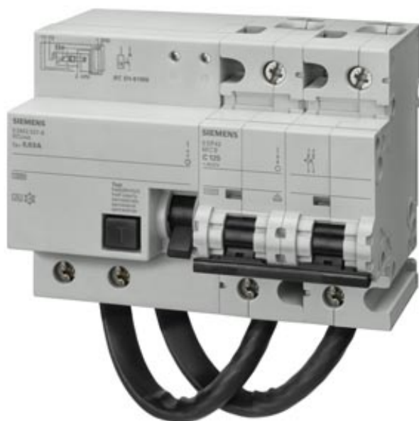
FI/LS-PROTECTOR TYP A (PSE), D=70MM IFN 30MA, 10KA, 2-POLEE B 125A
