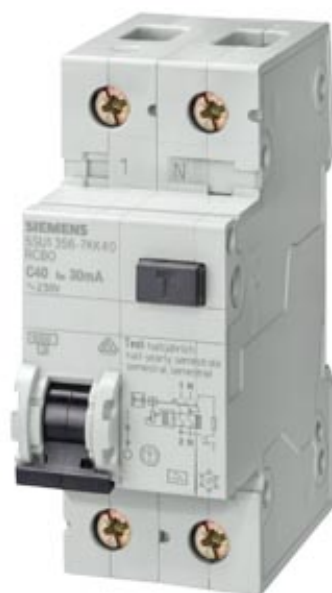
FI/LS-PROTECTOR TYPE A (PSE/SSF), D=70MM IFN 30MA,6KA, 1+N-POLEE C 40A
