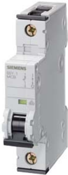
MINIATURE CIRCUIT-BREAKER UNIV. CUR. DC 220V AC 230/400V 10kA, 1-POLE, C, 25A FOR RAILWAY APPLICATIONS
