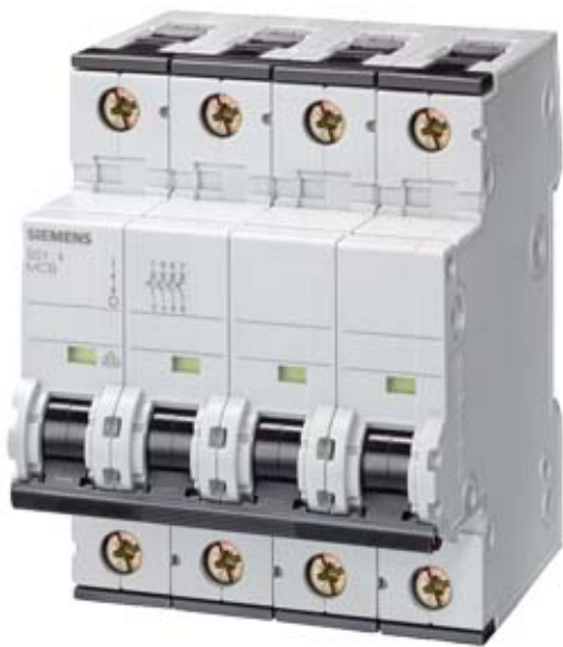
CIRCUIT BREAKER CURR.SENS.DC 880V AC 400V 10kA, 4POLE, C, 1.6A MAX. DC 1000V
